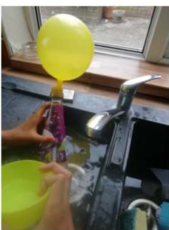
This is the bottle is cooled, it makes the balloon shrink because the air inside contract, this allows the air in the balloon makes its way into the bottle, hence the balloon shrinks.
