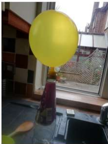
When the bottle is heated the air in it expands and pushes its way into the balloon, hence the balloon expanding.
