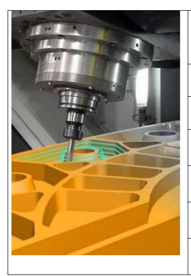
Most products that are needed in large quantities that are identical in size and need to be of an exact measurement are mass produced using Computer Aided Manufacture. CAM. Give some advantages and disadvantages.
